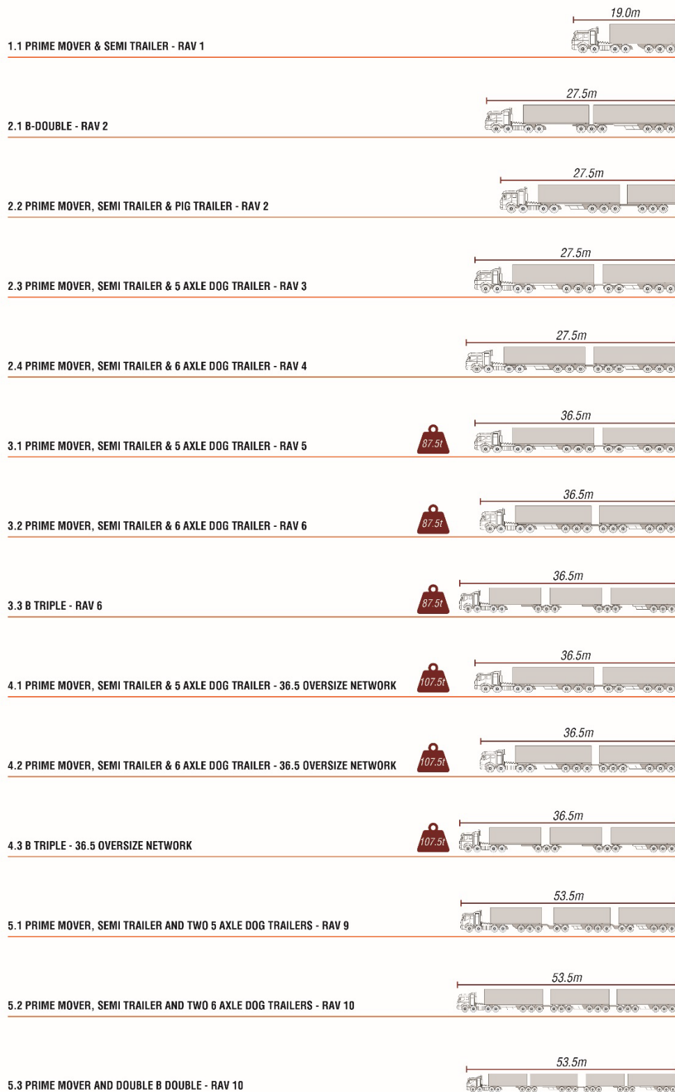
Figure 13 - MRWA classification of RAV networks and approved typical vehicles associated with each network
