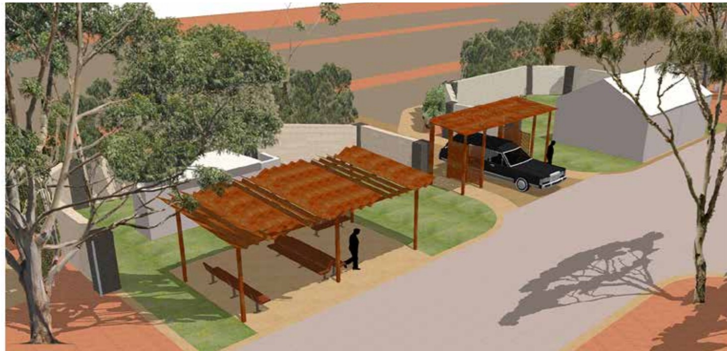
Shade Shelter at main entrance, axonometric view
