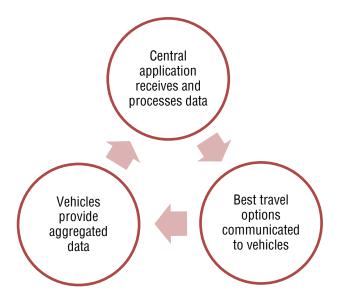
Vehicles need to be fitted with appropriate devices and software which would track speed, mass and position of the vehicle. Centralised system would use mass and speed related data for ensuring compliance (that heavy vehicles will stay on designated routes) while positioning will be used for tracking congestion, queues and travel times offering guidance to optimised legal access routes for heavy vehicles.
