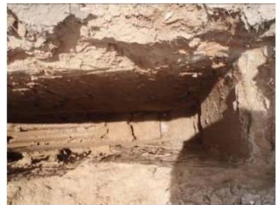
Photo 3: Testpit 1 bottom of hole. Termination due to water at 2.6 meters.
