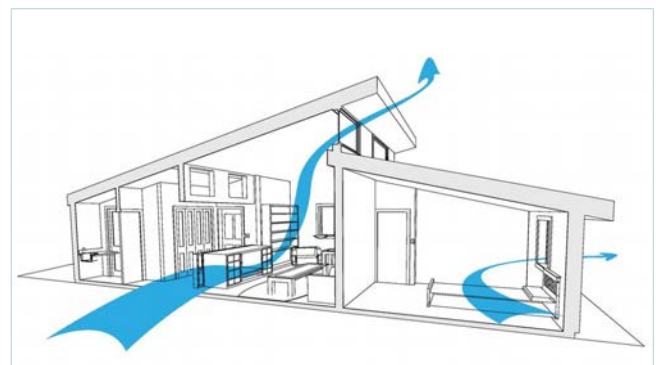
Smaller openings on the windward side of the building and larger openings on the leeward side will encourage the greatest ventilation through a space.
