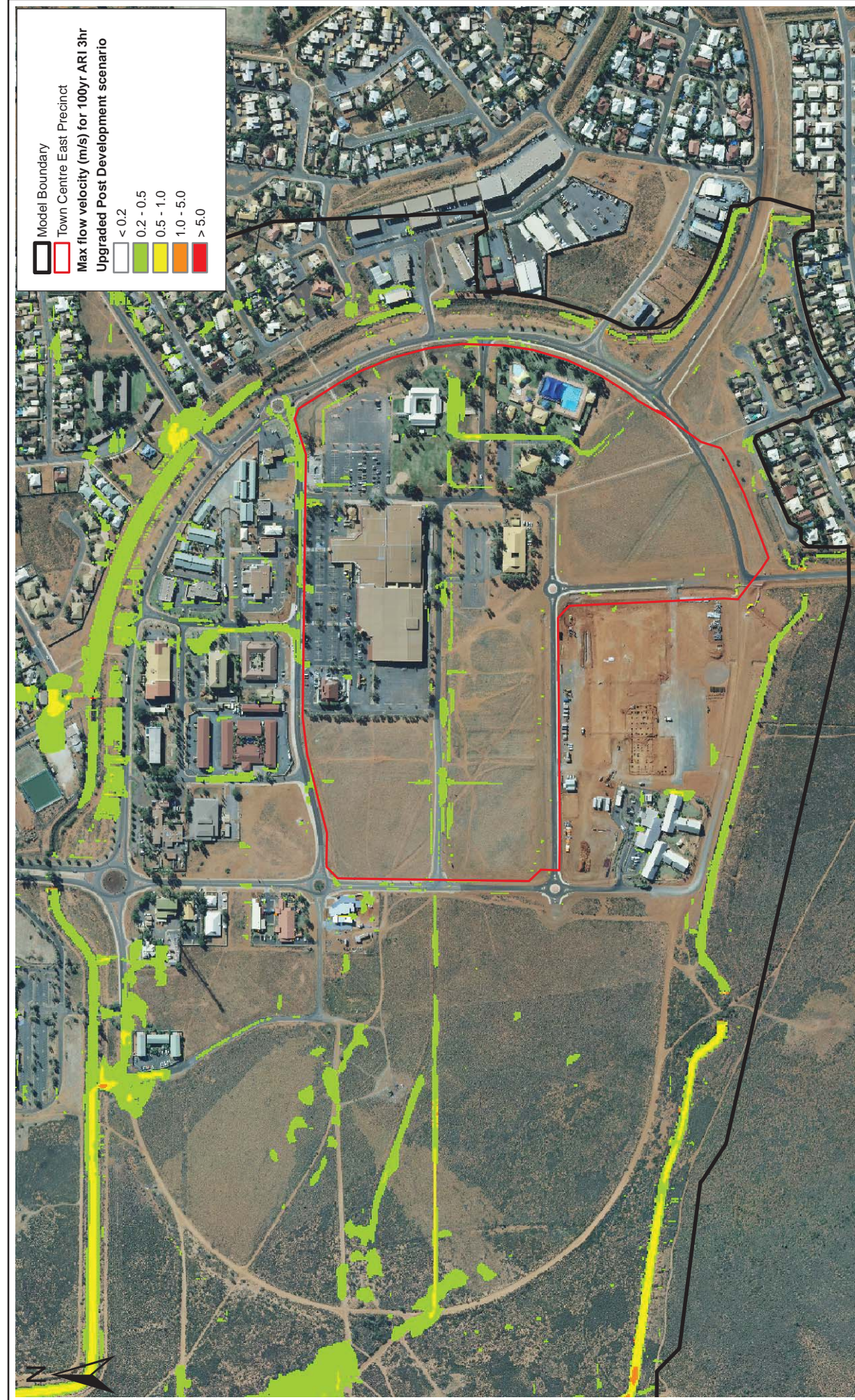
Landcorp South Hedland Town Centre Revitalisation: Flood Modelling Figure 33: 100 Year ARI 3 hour Event (Upgraded Post Development) Flow Velocities
