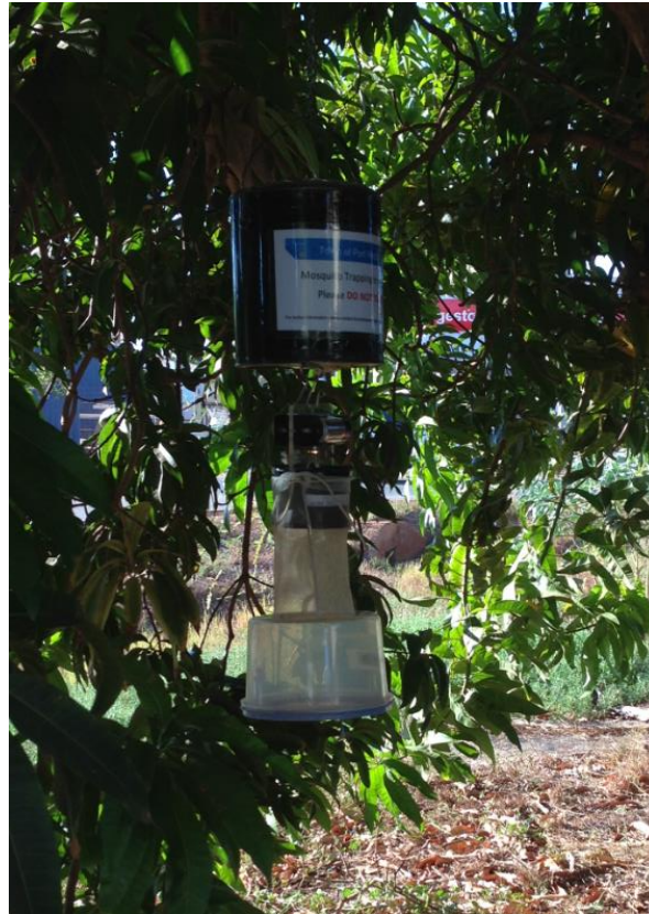
Figure 12. Light and Carbon Dioxide mosquito trap set up in sheltered area.
