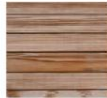
T1- SHIPLAP TIMBER CLADDING - STAINED FINISH
