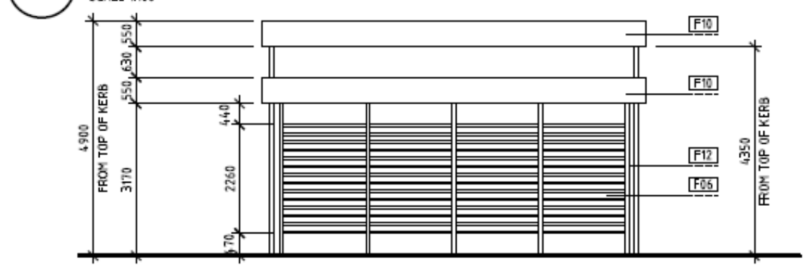
A DRIVE THRU CANOPY ELEVATION SCALE 1:100
