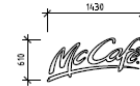
S4 BLADE SIGN S01 INDIVIDUAL HALO ILLUMINATED REVERSE PAN FABRICATED ALUMINIUM CHANNEL LETTERS. BRUSHED ALUMINIUM FINISH.
