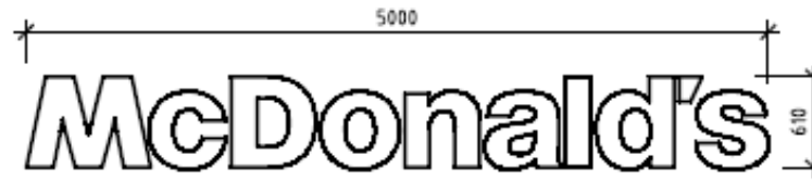
S2 WALL SIGN S01 INDIVIDUAL POLYCARBONATE LETTERING. INTERNALLY ILLUMINATED. WHITE LETTERS.
