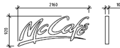
S4C WALL SIGN S01 INDIVIDUAL HALO ILLUMINATED REVERSE PAN FABRICATED ALUMINIUM CHANNEL LETTERS. BRUSHED ALUMINIUM FINISH.
