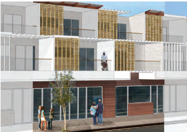
A mixed-use building concept responsive to the Pilbara with room sized balconies, permeable balustrade and roof to maximise the opportunity to purge hot air.
