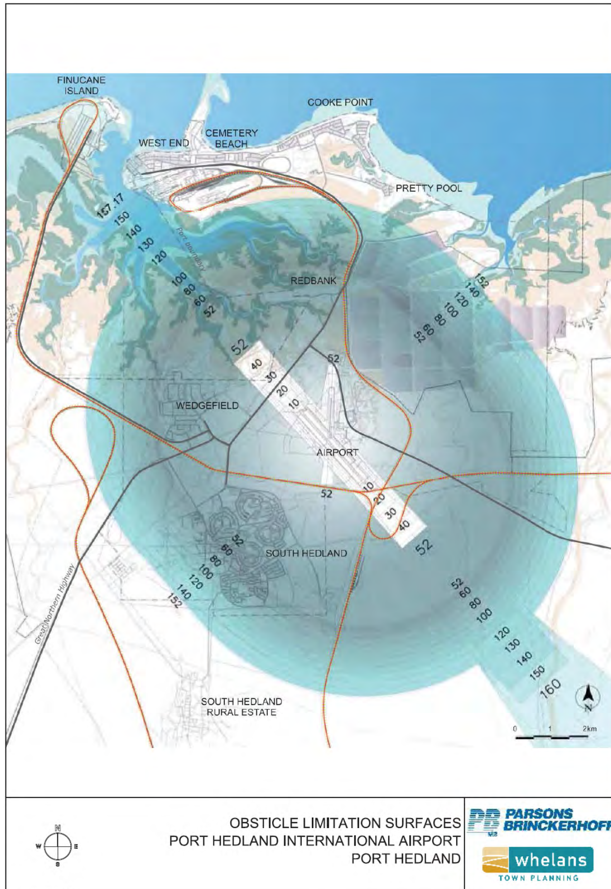
Figure 6. Obstacle Limitation Surfaces (Source: LUMP)
